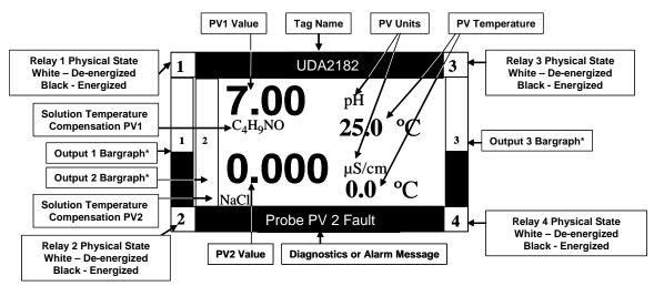
\*On the display, the bargraphs are the outputs in Engineering Units, the corner annunciators are the physical relay states.
